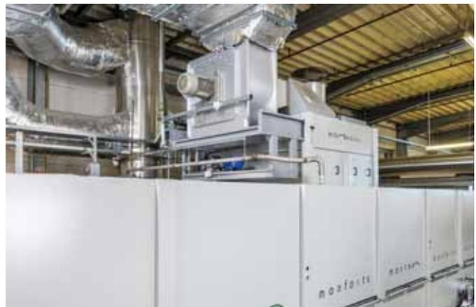
T-CA solution of combined reactive and disperse dyes in particular, the improvement in both dyed fabric quality and dye fixation is considerable, and with significant savings in energy and time due to the combined bleaching and padder fixation.
