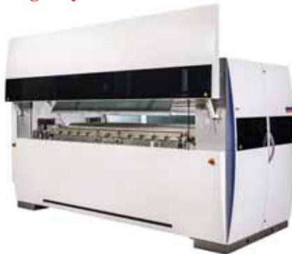
The latest singeing machine is equipped with two burners and a double nozzle strip – 100% made in Germany. The silicium carbide burning chambers ensure complete combustion, and a constant burner temperature thanks to four cooling channels. Low gas consumption and a perfect flame will increase the scope of fibres and blends.
