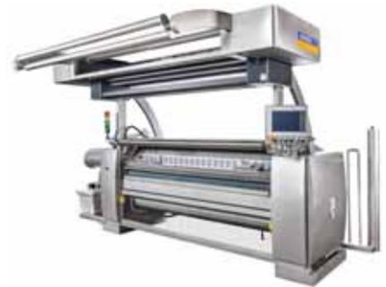
The heart of the CPB dyeing station is still the padding mangle with two Küsters S-roller systems. Now it offers best accessibility through optimised design with compact dimensions and a dyeing trough that swivels downwards and backwards. Enhanced operator safety is another key feature of the new design. Benninger is the market leader for 100% level dyeing results with no listing or tailing. The S-roller technology creates a nip profile adapted perfectly to the fabric and process requirements.
