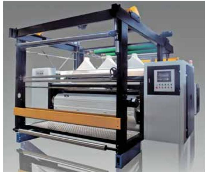
type machine come with two different workings one is manual and another one is PLC controlled machine. In manual control machine to change speed of pile and counterpile rolls we need to change the gear of rolls but in PLC control machine these speeds can be adjusted by PLC and Inverters.
