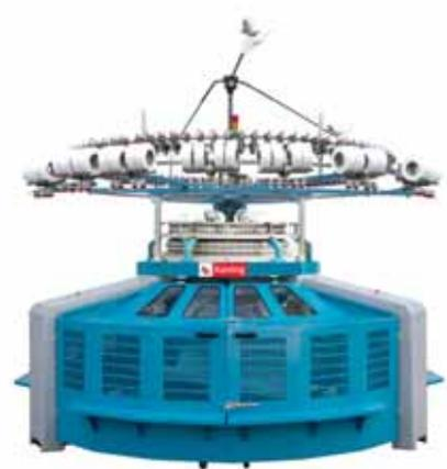
and ground in the CNC machine, which makes the needle track smooth and the needle durable while machines run at high speed. The streamlined cams are easy to adjust which also makes the needle smooth and stable at high speed.
