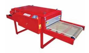
chamber. The Solutions dryers feature the same double-wall construction as Anatol's gas dryers, re-enforced with high-efficiency thermal insulation. Solutions Series electric dryers offer programmable temperature controls with automatic cooldown. Solutions electric dryers are available in six configurations, with four basic models, from 24" belts with 4' of heat up to 60" belts with 10' of heat.
