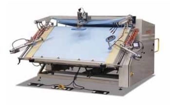
2. Pressing and drying on the pressing plate, steam heated, steaming and with vacuum.
